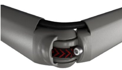
7) bionic tendon and hidden cable conduits in the arms
