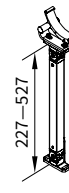
raised cassette bracket foot can be tilted backwards by up to 45°, head of cassette fixture bracket can be tilted forwards by up to 45°
