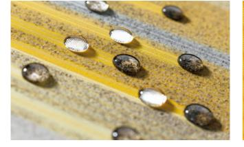
Self-cleaning snc effect Water droplets pick up dirt particles and run off the awning cover (the awning must be set at a pitch of at least 14 degrees). This gives you the peace of mind that your fabric will retain its colour and vibrancy for years without you having to lift a finger.
