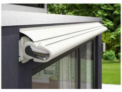
**Wall sealing profile** The slim aluminium profile in the awning colour closes the gap between the awning and the wall, allowing rain to be discreetly drained off the awning.
